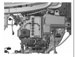
3. Battery in the engine compartment
