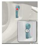
1. Pull the release lever 1 to unlatch the hood. The hood should pop open slightly.
