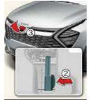
2. Raise the hood slightly, push the secondary latch up
