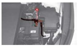
b) Remove the PE room junction box cover (A).
