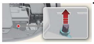
If the charging cable does not detach due to battery discharge and failure of the electric wires, open the hood and slightly pull the emergency cable as shown above. The charging connector will then unlock.
