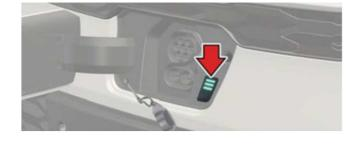
The battery charge status indicator (3 separate lights),located inside the charging door, is illuminated when the vehicle is charged. The number of lights illuminated indicates the charge level of the battery.
