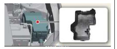
Engine room fuse box ※ The actual engine room in the vehicle may differ from the picture.
