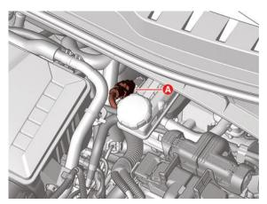
b) Remove the service interlock connector (A).
